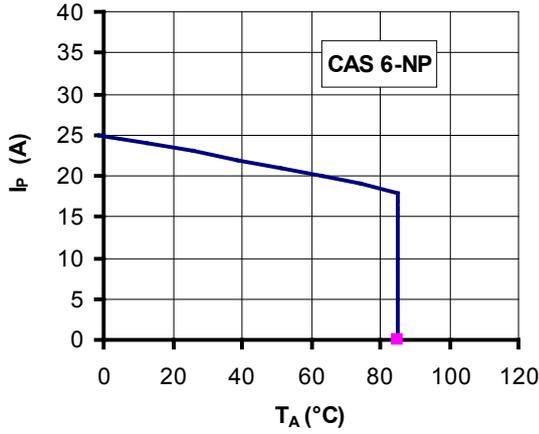
Figure 25: I<sub>p</sub> vs T<sub>A</sub> for CAS 6-NP
