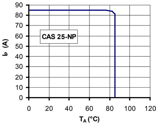
Figure 27: I<sub>p</sub> vs T<sub>A</sub> for CAS 25-NP
