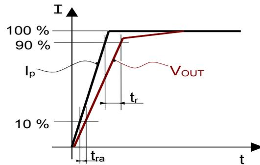
Figure 31: Response time  $t_r$  and reaction time  $t_{ra}$
