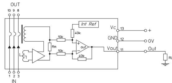
Figure 32: Test connection
