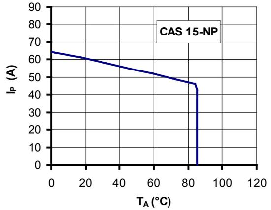
Figure 26: I<sub>p</sub> vs T<sub>A</sub> for CAS 15-NP
