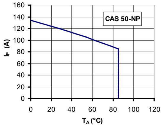
Figure 28: I<sub>p</sub> vs T<sub>A</sub> for CAS 50-NP
